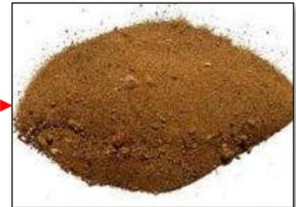
**AFTER** – Drill cuttings after being processed by a VCD.
